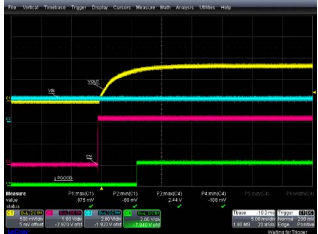
FIGURE 16. POWER-ON AND POWER-OFF, EN = 0 TO 1, +25 °C, VIN = 2.2V, VOUT = 0.8V, IOUT = 0.5A, PGOOD TURN-ON
