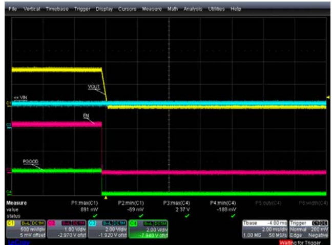
FIGURE 18. POWER-ON AND POWER-OFF, EN = 1 TO 0, +25 °C, VIN = 2.2V, VOUT = 0.8V, IOUT = 0.5A, PGOOD TURN-OFF
