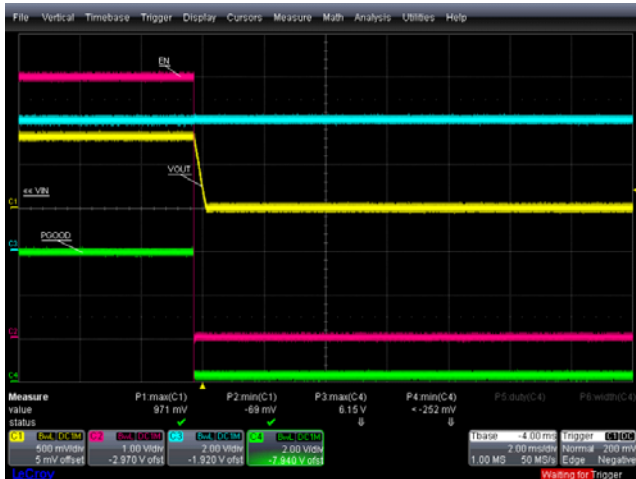
FIGURE 17. POWER-ON AND POWER-OFF, EN = 1 TO 0, +25 °C, VIN = 6V, VOUT = 0.8V, IOUT = 0.5A, PGOOD TURN-OFF
