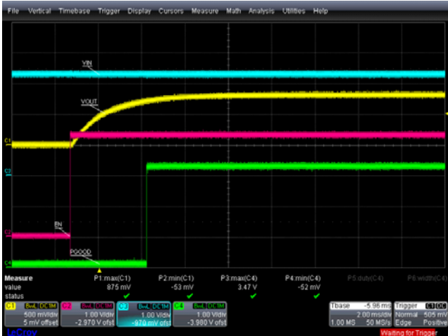
FIGURE 15. POWER-ON AND POWER-OFF, EN = 0 TO 1, +25 °C, VIN = 6V, VOUT = 0.8V, IOUT = 0.5A, PGOOD TURN-ON
